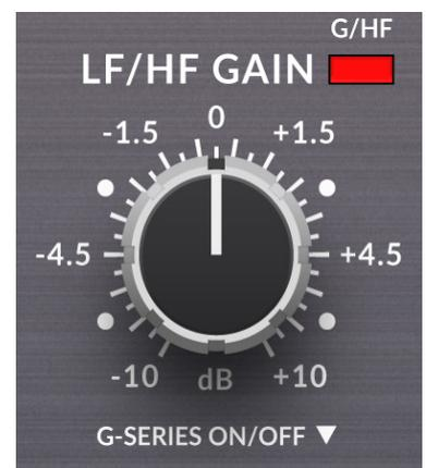
*Red LED indicates the control functions as HF GAIN*
