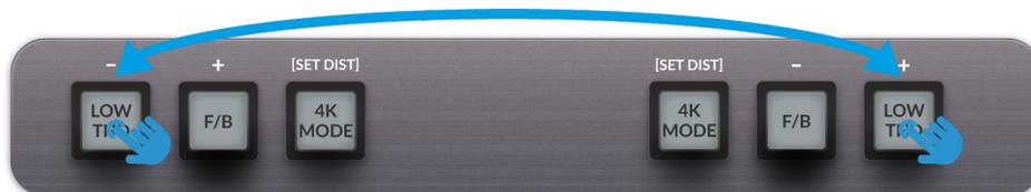
*Press and hold both LOW THD switches during boot until central switches start flashing, then release.*
