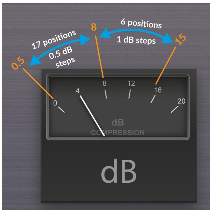
*For example, the needle is showing that the Range is set to 4 dB here.*
